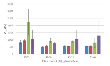
Figure 3: Average  $P_{cap}$  with increasing fiber content. From left to right for each fiber content: glass warp, glass weft, carbon warp, carbon weft.
