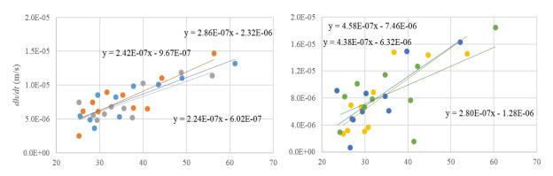
Figure 1: Example linear fits of Equation 1, for uncompressed carbon warp (left) and weft (right) flow directions.
